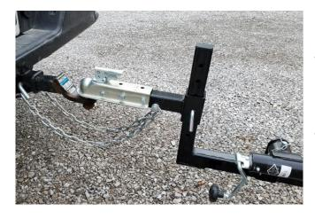
Connect the sweeper to the tow vehicle with the 2" ball coupler and safety chains. You must use a 2" Trailer ball, unless you purchased an optional Pintle Ring.
