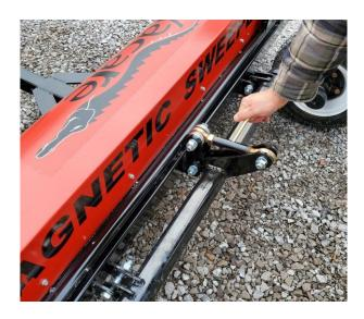
Adjust the sweeping height (distance from ground to bottom of sweeper) between 2" and 5". The lower the better, but make sure magnet is not constantly hitting the ground.
