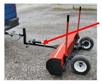
The tongue of the sweeper should be as level as possible. This can be adjusted by changing the position of the coupler on the trailer tongue or the ball mount on the tow vehicle.
