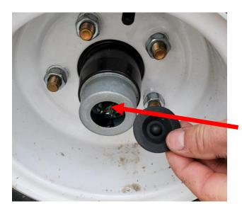
Remove rubber cap and using a grease gun apply wheel bearing grease to the grease nipple in each wheel hub once per year.
