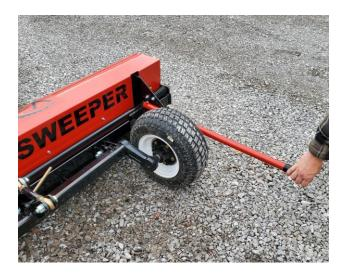
To clean debris off of the magnet. Stop the tow vehicle. Push Down on the release handle until the handle stays in the down position.
